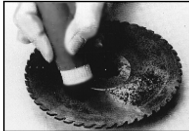
Rust and Corrosion Removal
