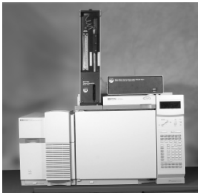
Figure 2 - Desorption Unit mounted on an Agilent 6890 GC
