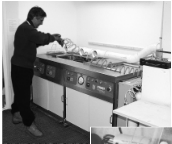
Parts are thoroughly cleaned in solvents and rinsed in a state-of-the-art ultrasonic aqueous cleaning system.
