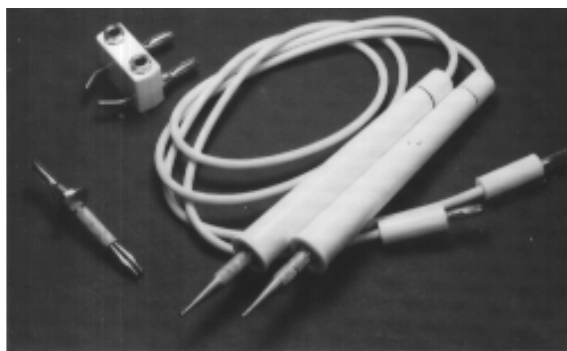
Auxiliary cables, annealing jack, and plug-in vise
