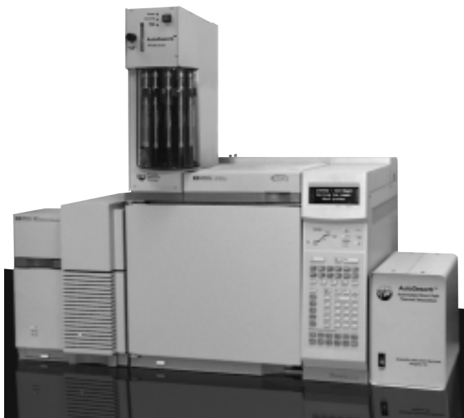
AutoDesorb System mounted on the Agilent 6890 GC and 5973 MSD
