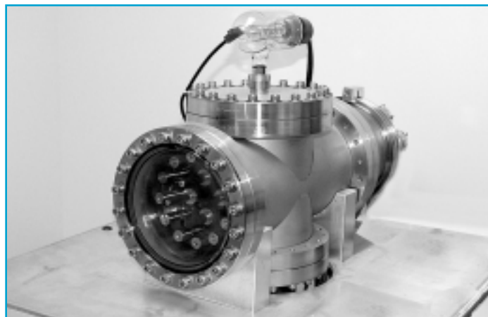
Figure 2 - SIS Filament Testing Station
