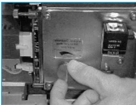
Vent the instrument. Make sure that all voltages applied to the multiplier and the conversion dynode are turned off prior to venting the system.
