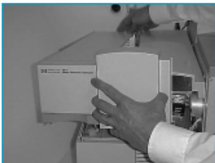
Remove the top cover of the Mass Spectrometer
