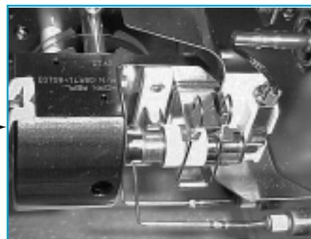
Remove power and computer cables from the Mass Spectrometer. Swing the Mass Spectrometer door open and locate the electron multiplier region.
