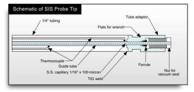
for the outer probe shaft, however, the end of the probe is fitted with a tube adaptor, stainless steel ferrule and nut which when tightened provides the vacuum seal around the capillary tubing. To replace a clogged capillary, use a tube cutter to cut the capillary at the back of the probe, loosen the nut, slide out the 1/16" clogged capillary, and insert a new capillary. The thermocouples are spotwelded to the inner guide tube into
