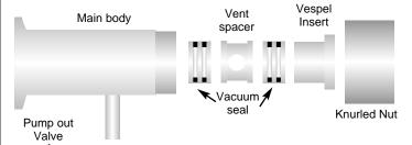
SIS has redesigned the probe inlet system for the HP Engine. This new port has two major improvements. The first improvement is in the probe sealing
