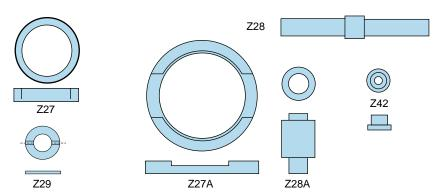
Several new ceramic insulators are now available for the Finnigan MAT Ion Trap in addition to the ceramics listed in our catalog. All ceramics are constructed from high purity alumina ceramic. In addition the ceramics kit for the ITD is also available. This kit consists of two gate insulators (Z27A) and six position pins (Z28A). For other ceramics or special requirements of ceramic insulators call us with your requirements.
