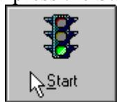
on the right side of the ProbeDirect main display panel. The green “Start” button on the front of the Probe Controller performs the same function. Note that the “Status” panel must show “Connected” for the program to begin. Other processes, such as Cooling, must be stopped before a new program can be started.
