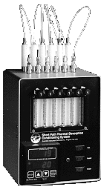
Figure 23 Thermal desorption tube conditioning oven
