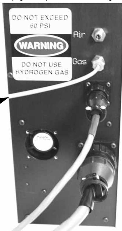
Figure 20 - Attaching Carrier Gas Line to back of AutoDesorb Tower
