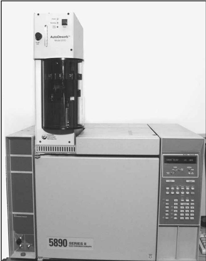
Figure 33 - AutoDesorb system mounted on top of 5890 GC
