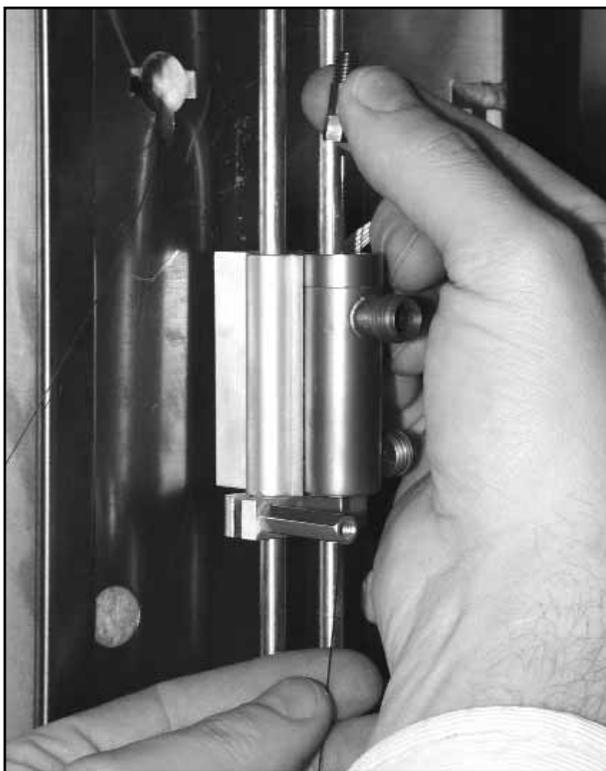
11. Connect the cryogen supply tube to the outlet of the appropriate valve. When using LN<sub>2</sub>, insulate the valve body and the length of tubing that runs from the valve to the oven wall. Plumb the valve to the cryogen supply.
