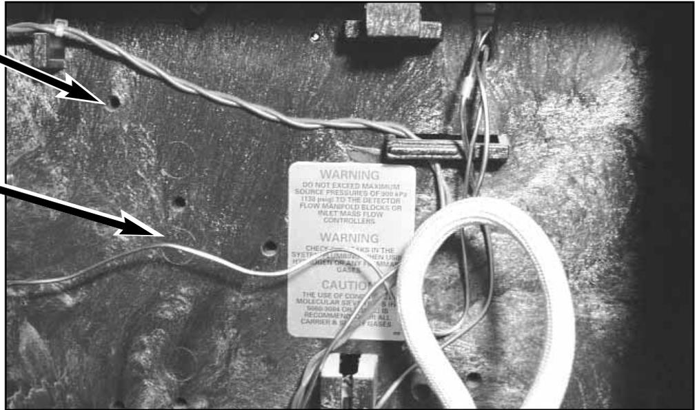
Figure 23 - Left side of 5890 GC - Locating Carrier Gas Line
