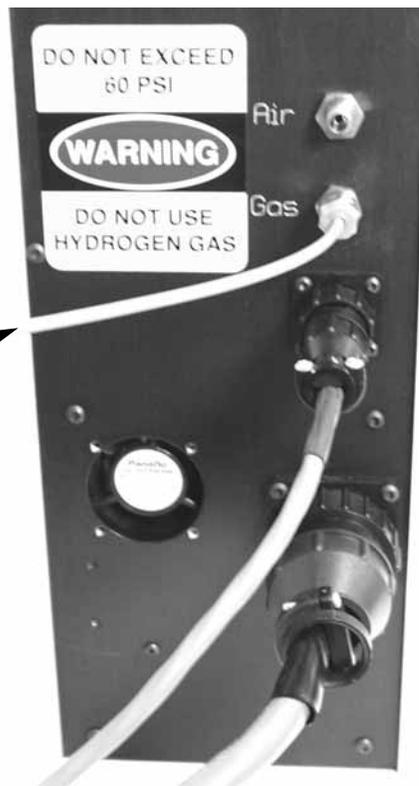
Turn on the carrier gas to the instrument, pressurize the front inlet, and check all plumbing connections for leaks.
