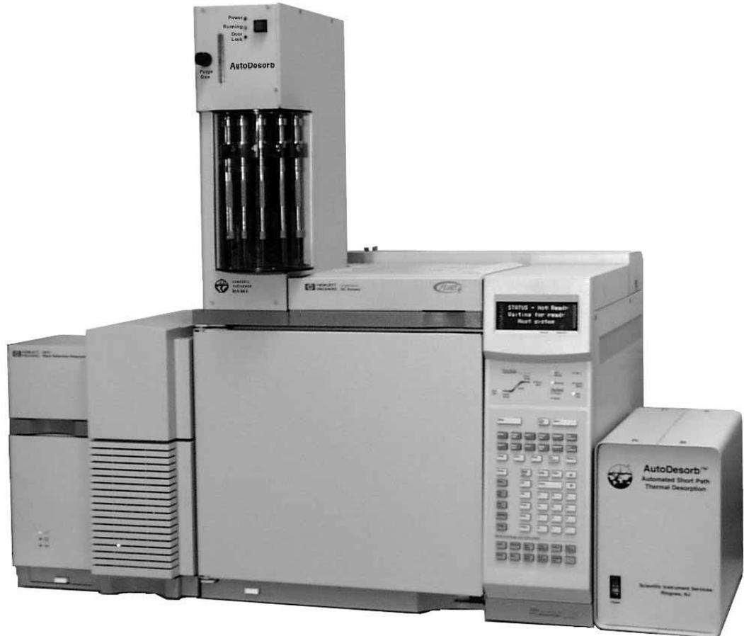
**Figure 21 - AutoDesorb Installed on the 6890 GC with 5973 MSD**
