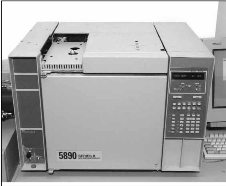
Figure 32 - Baseplate and new front plate installed on 5890 GC
