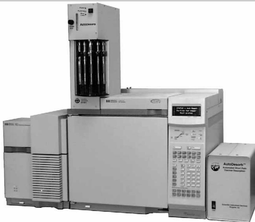
**Figure 5 - AutoDesorb mounted on Agilent 6890 GC and 5973 MSD**
