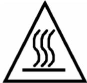
Temperatures up to 450°C are present inside the desorption unit under normal operating conditions. KEEP HANDS AND FINGERS OUTSIDE OF THE DESORPTION UNIT.
