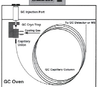
Micro Cryo-Trap Mounted Inside GC Oven
