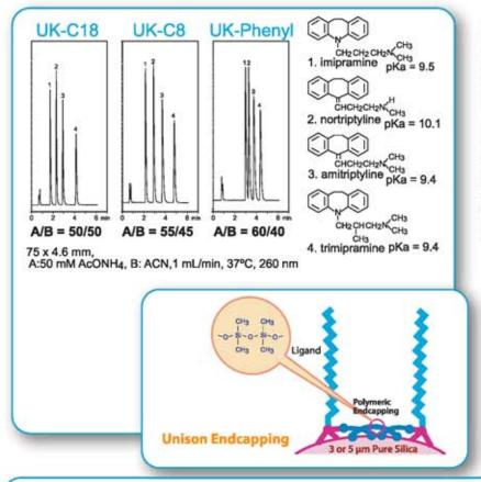
Unison employs a unique endcapping technology. As a result, the column provides excellent elution characteristics for difficult separations, such as that of basic compounds. This applies not only to ODS, but also C8 and phenyl columns.
