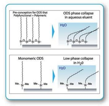
Conventional ODS silica phases, which are designed for the separation of polar compounds, usually have lower coverage than silica stationary phases. This is necessary to avoid phase collapse.
