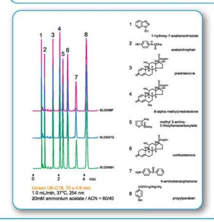
This data shows the exceptional batch-to-batch reproducibility for Unison UK-C18, a column packed with high efficiency 3µm C18 silica particles.
