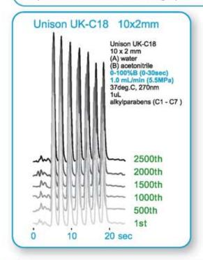
For superior throughput, utilize Unison's high efficiency and use a shorter column. Many customers have cut their run times drastically by using our 10mm, 20mm, and 30mm column lengths, while still achieving satisfactory separation. All of these column lengths come with 3µm silica packing material. We advise our customers to test increasingly shorter columns until they find the optimal trade-off between speed and separation.
