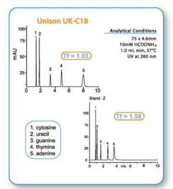
Nucleic bases, especially adenine, frequently give poor peak symmetry on commercial ODS columns under hydrophilic conditions.
