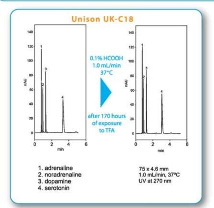
Formic acid is important for LC-MS. The new ODS phase, Unison UK-C18, showed excellent stability for catecholides after 170 hours of exposure to 0.1% TFA.
