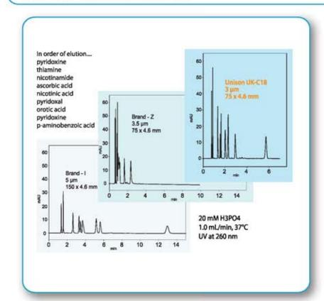
Hydrophilic vitamins are important analytes and require aqueous eluent under acidic conditions for optimized separation.
