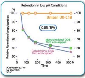
Our studies show that trifunctional, TMS endcapped stationary phases provide greater stability under extreme acidic conditions (pH 1.5) when compared to traditional monofunctional ODS TMS endcapped columns.
