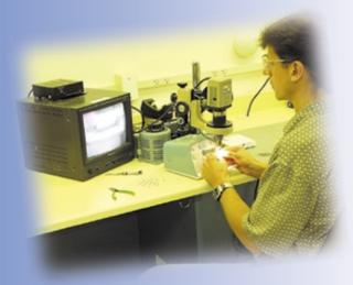
Precision spotwelders are combined with custom designed and manufactured electrodes and fixtures to maintain accuracy and precision on all the filaments we manufacture. Microscopes are mounted over many of our spotwelders to provide additional accuracy. In some cases video systems are utilized to assure accurate manufacture of our filaments.
