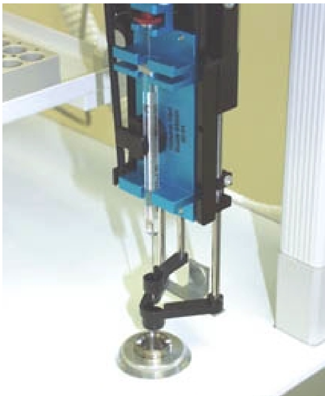
Figure 25 - CTC PAL Autosampler Syringe injecting sample
