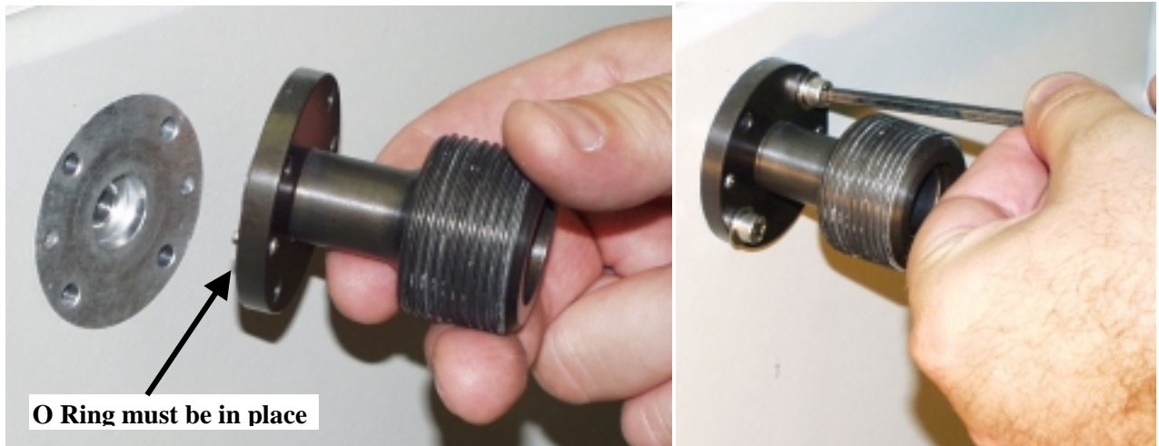
Figure 84 - Attachment of Inlet Assembly Coupling
