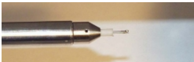
Figure 32 - Remove the Source Calibration Tip and Install the DEP Filament Probe Tip
