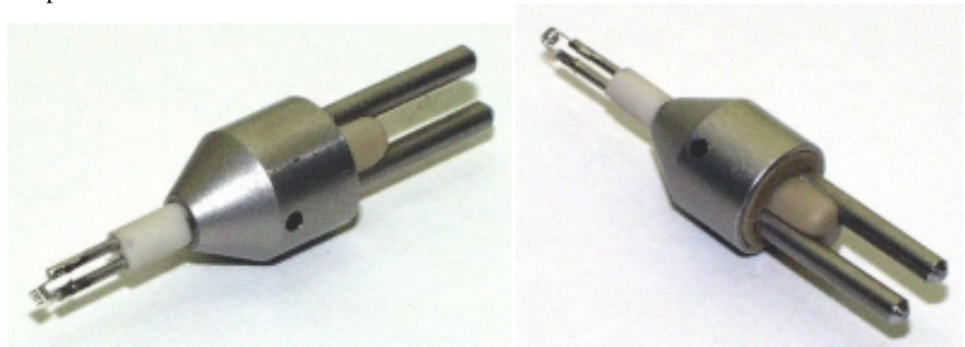
Figure 57 - Front and Back Views of Plug- In DEP Probe Filament
