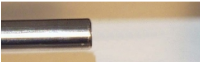
Figure 56 - Probe Shaft with DEP Probe Filament removed
