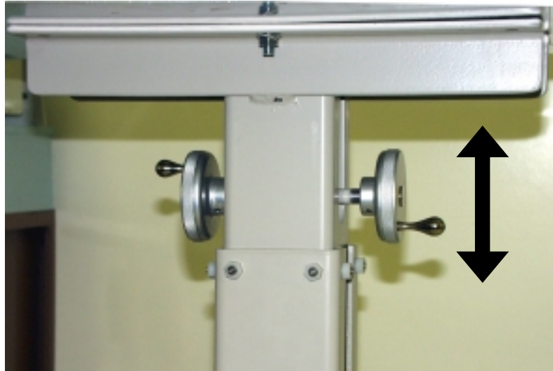
Figure 16 - Crank handles permit AutoProbe height adjustment
