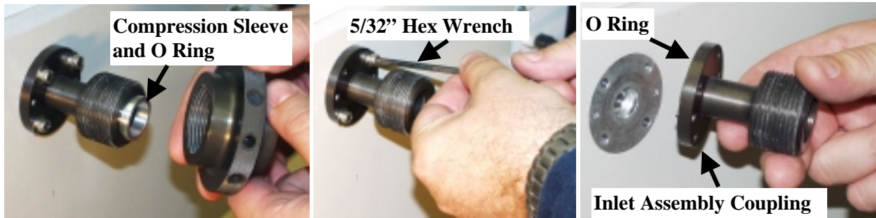
Figure 59 - Removing the Inlet Assembly Coupling
