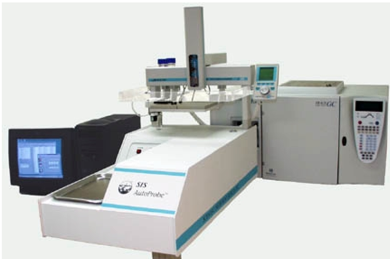
Figure 1 - AutoProbe attached to the Thermo Finnigan TRACE MS
