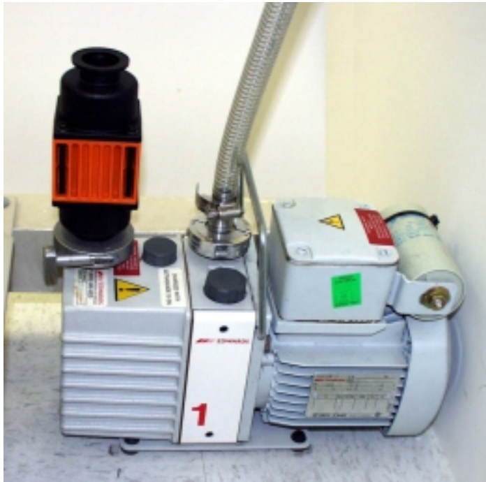
Figure 88 - Rotary Pump for the evacuation of the pump isolation valve
