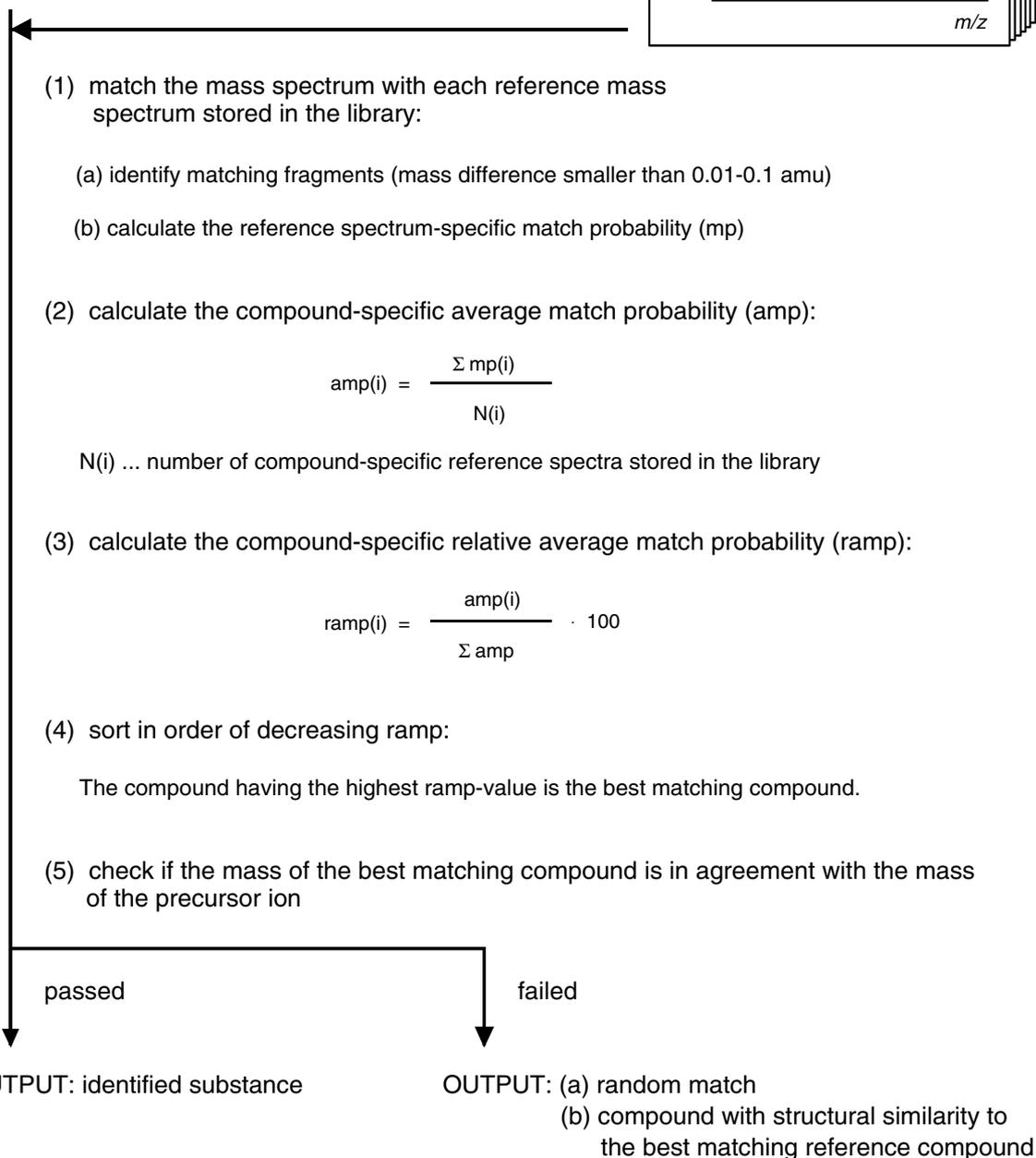
**Figure 1.** Schematic drawing showing the principles of the automated database search approach. Details are described in the text.
