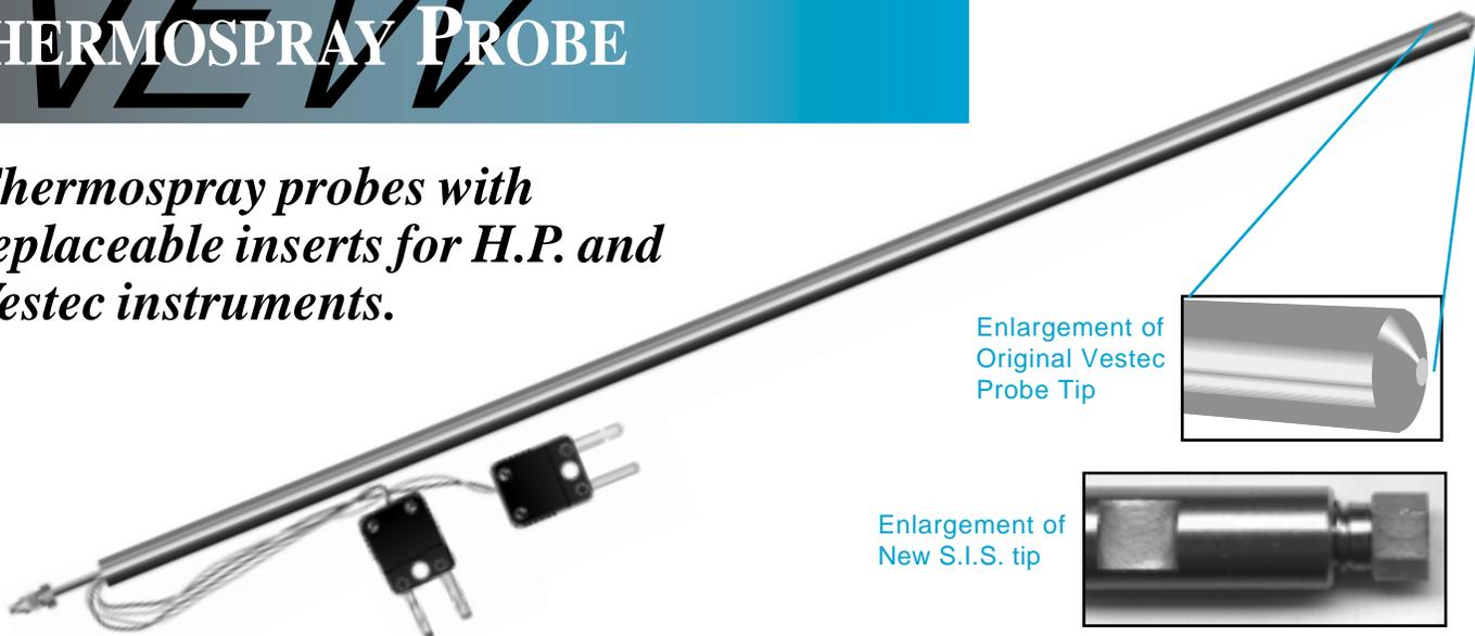
Scientific Instrument Services has redesigned the Vestec thermospray probes so that the capillary inserts can be quickly and easily replaced by the user when necessary. Clogging problems with the original vestec thermospray probes is well documented. The original probes when they became clogged were virtually impossible to unclog and therefore the probe had to be sent back for repair or be replaced completely.
