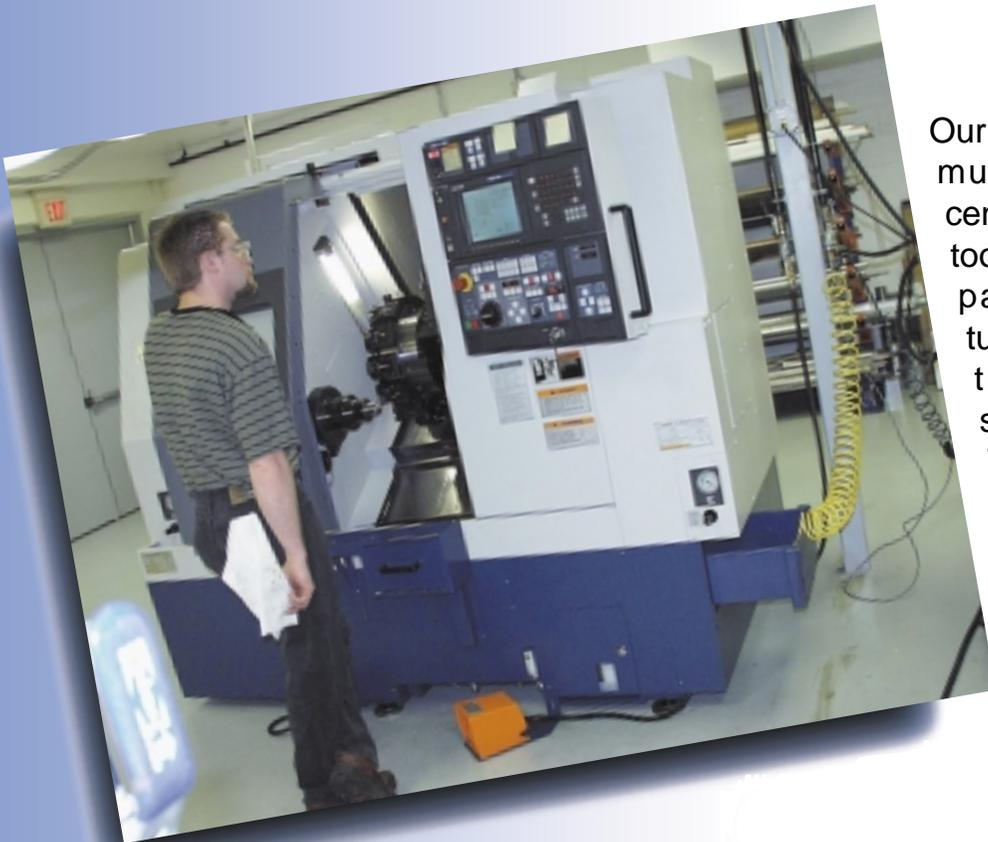
Our turning capabilities include a multi-axis Mori Seiki turning center with sub spindle and live tooling. This allows for complex parts that not only include turning, but milling, drilling and threading to be done in a single, unattended operation. This minimizes part handling and setups and provides the utmost in accuracy and precision.
