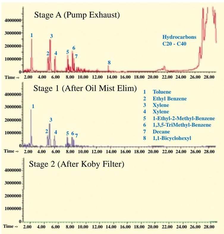
Figure 1 - Efficiency of Vacuum Pump Exhaust Filters
