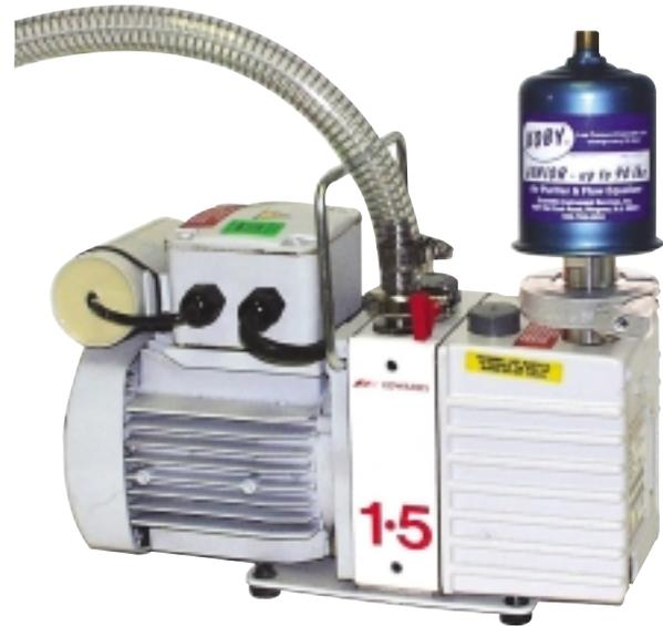
The Koby air purifier is normally used in conjunction with an oil mist eliminator. However, the Koby air purifiers can be mounted directly on top of the exhaust port on the vacuum pump as shown above. In other systems where space is limited, it is more convenient to attach a hose to the pump exhaust port and then adapt the Koby air purifier to fit the vacuum hose. (See SIS Catalog or Web site for additional details)
