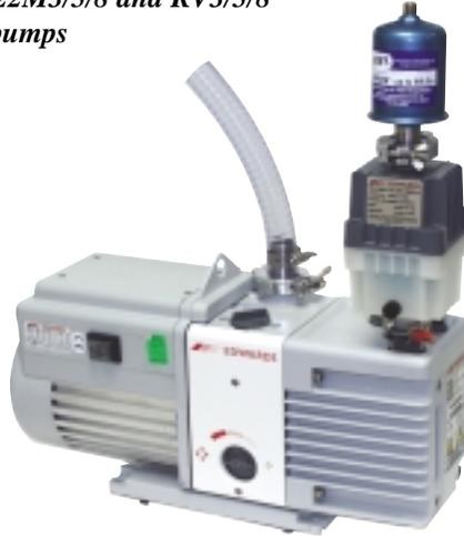
The Pump Filter Kit for the Edwards Pump includes the Edwards EMF10 Oil Mist Eliminator, Koby Charcoal Trap and all fittings needed to attach this two filter system on the larger Edwards vacuum pumps. This kit is to be used with Edwards models E1M5/8, E2M2/3/5/8 and the RV3/5/8 vacuum pumps. It can also be used with any other manufacturers pumps that have an NW25 flange type fitting on the exhaust port.
