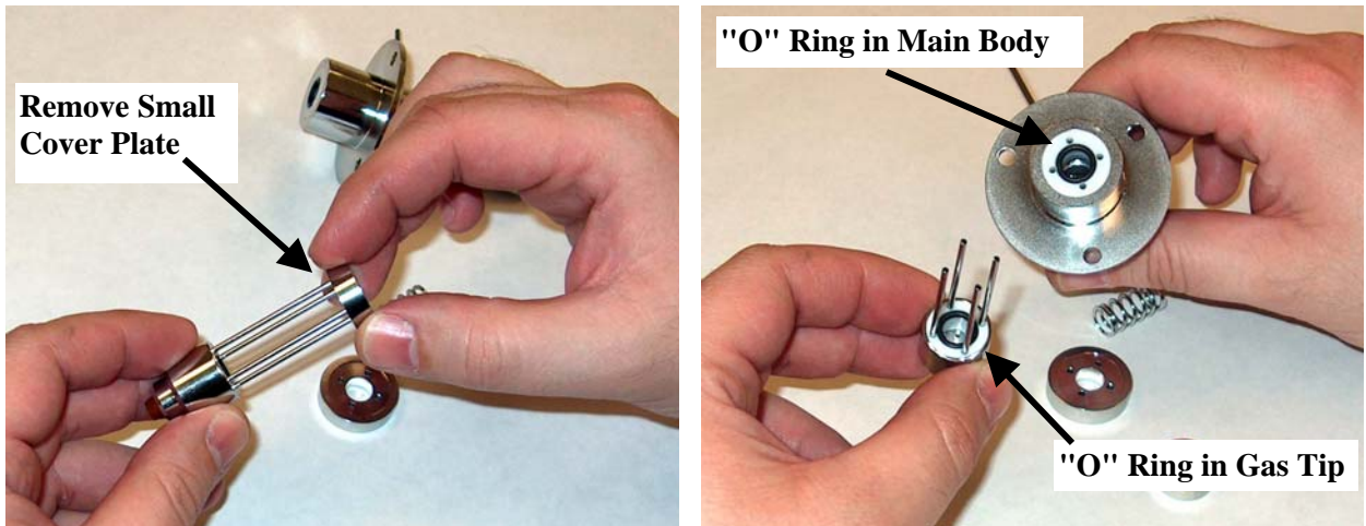
Figure 91 - Removal of cover Plate to access the "O" Rings in the Transfer Line
