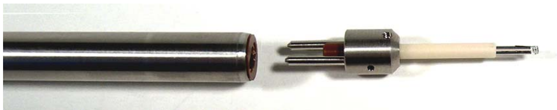
Figure 52 - Probe Shaft with DEP Probe Filament removed
