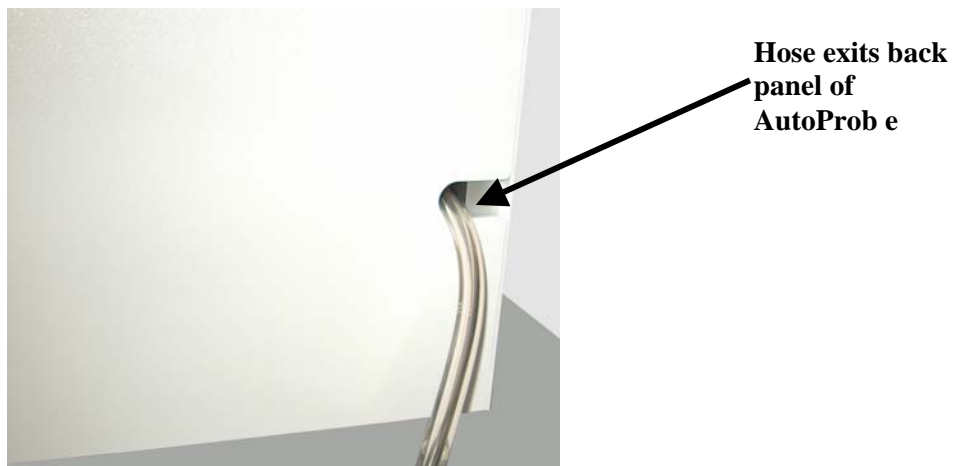
Figure 20 - Installation of the Vacuum Pump Hose to AutoProbe
