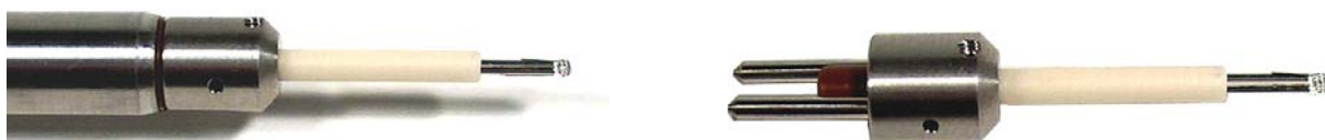
Figure 2 - DEP Probe Tip
