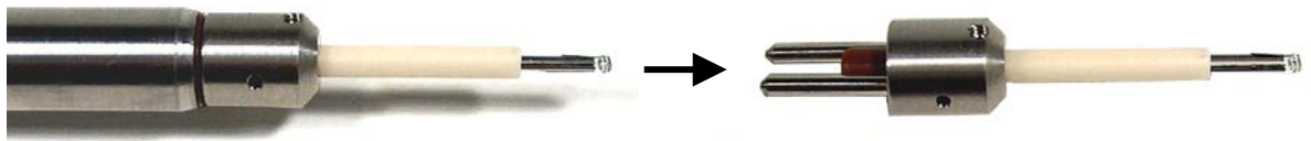
Figure 51 - Replaceable DEP Probe Filament
