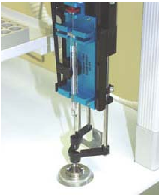
Figure 22 - CTC PAL Autosampler Syringe injecting sample
