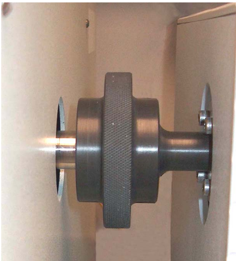
Figure 17 - AutoProbe attached to the MS with Compression Nut
