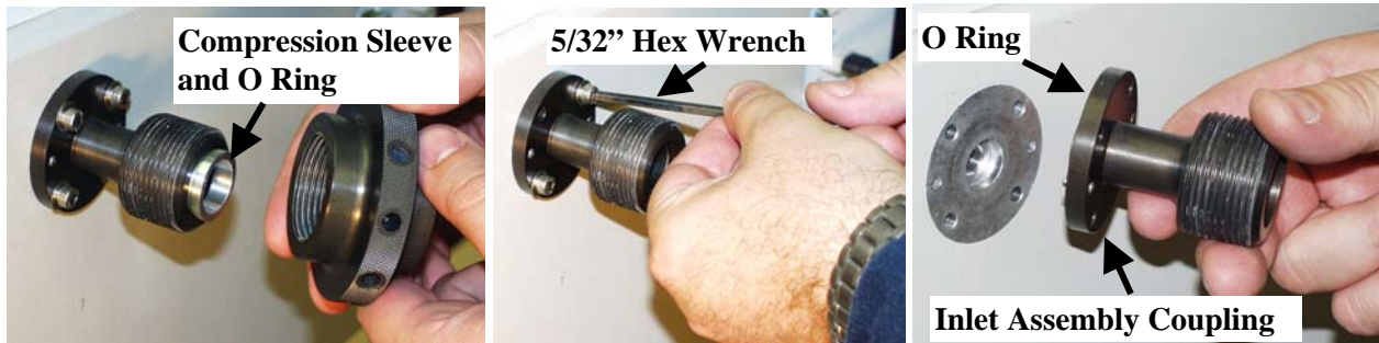
Figure 55 - Removing the Inlet Assembly Coupling
