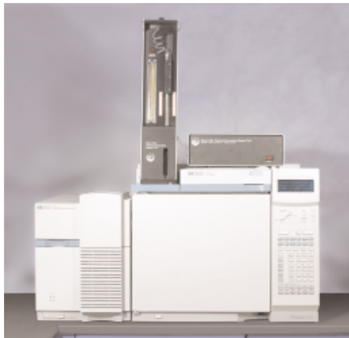
Figure 2 - Desorption Unit mounted on an Agilent 6890 GC
